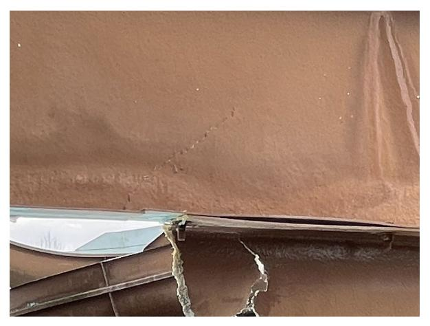
Previously repaired damage to a splash guard panel immediately downstream from the failed panel is noted. The area around two bolt locations is ripped out and has been patched to provide material for the bolt attachment.
